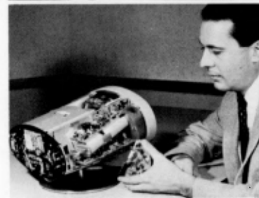
The invention of the transistor in 1948 by a team of Bell Labs scientists helped make possible the compact size of the Picturephone instrument.
